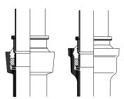
Adaptors are also available to connect Rainwater downpipes to underground drainage systems of other materials.
