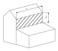
For a single wall the effective catchment area is taken to be half the area of the elevation.  $E = \frac{1}{2} \left( \text{Li} \times \text{Hi} \right) \text{m}^2$
