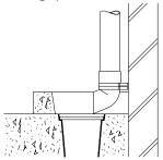
Alternatively the rainwater can discharge into a back inlet gully through an adaptor and bend.
