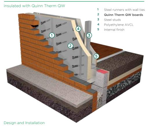
Quinn Therm QW boards should be butted tightly together to form a continuous layer of insulation. The boards should be cut to fit tightly to the back of door and window framing. Any gaps between the insulation and framing should be filled with expanding polyurethane foam.
