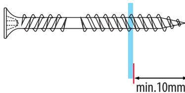
In order to guarantee a secure fixing, the screw must fully penetrate and protrude through the back of the steel by a minimum of 10mm
