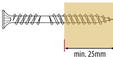
In order to guarantee a secure fixing, the screw must fully penetrate any supporting timber by a minimum of 25mm
